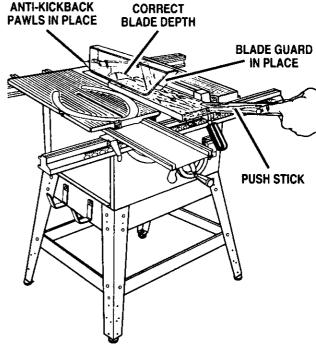
NO KNOTS, NAILS OR WARPS IN WOOD, WOOD FED AND SUPPORTED CORRECTLY
